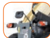
Rear Road Lights
